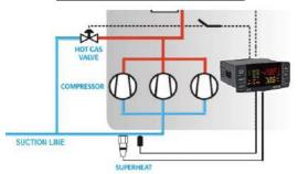
To detect the suction superheat an auxiliary probe among P3 (term. 3-4) or P4 (term. 27-28) has to be set as superheat temperature probe.
