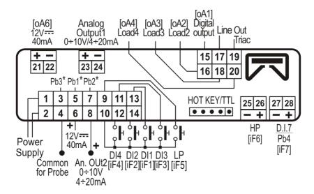
Power supply: model at 12Vac/dc supply: use terminals 1-2 Power supply: model at 124Vac/dc supply: use terminals 1-2
